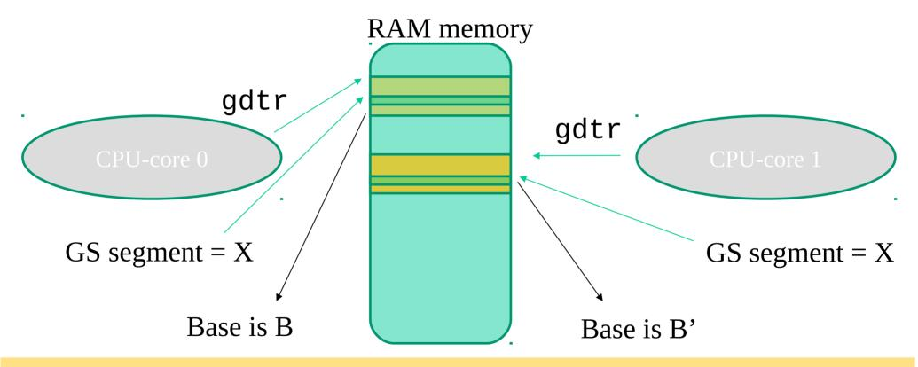
Same displacement within segment X seamlessly leads the two CPU-cores to access different linear addresses
