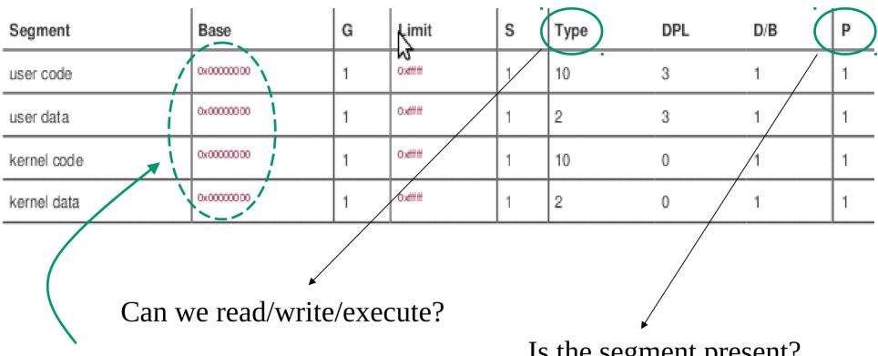
x86-64 directly forces base to 0x0 for the corresponding segment registers
