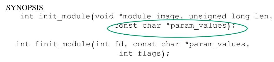
Note: glibc provides no header file declaration of init\_module() and no wrapper function for finit\_module(); see NOTES.
