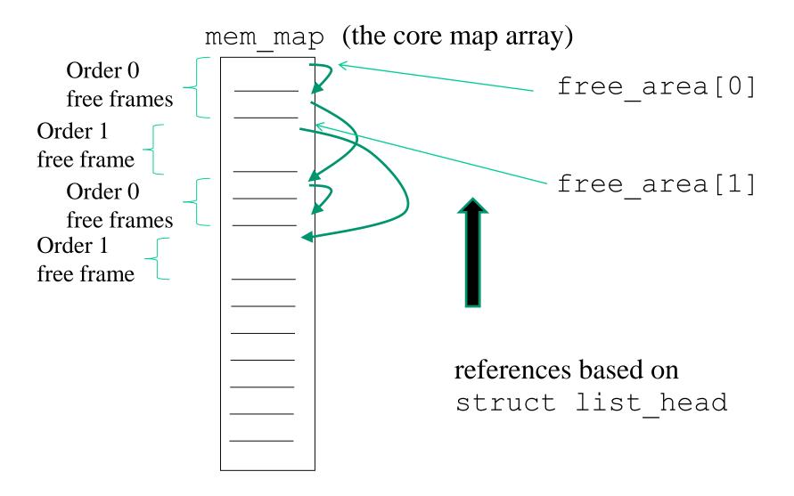
Recall that spinlocks are used to manage this data structure
